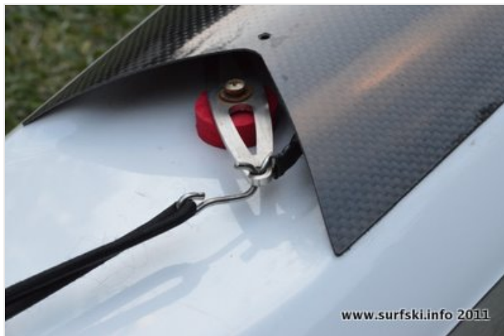
The bungi has a blunt stainless steel hook on the end - hooked here onto the tiller bar
