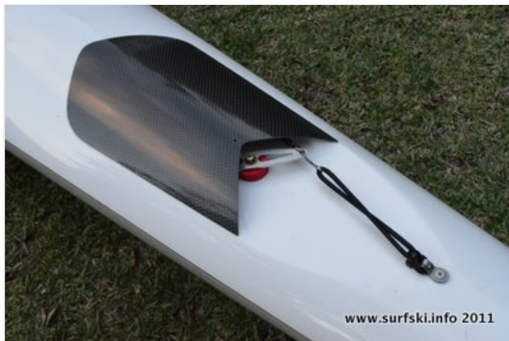
The left hand rudder line has snapped; the emergency steering system is now hooked to the right hand end of the tiller bar. Steering is now possible using the right hand rudder pedal only.
